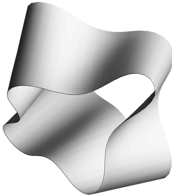
Fig. 6. Postcritical equilibrium configuration of the cylindrical shell compressed by four radial forces.
